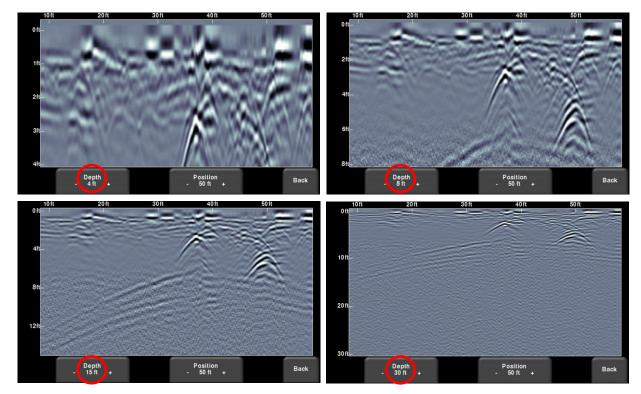
Figure 8-6: Varying displayed depth
