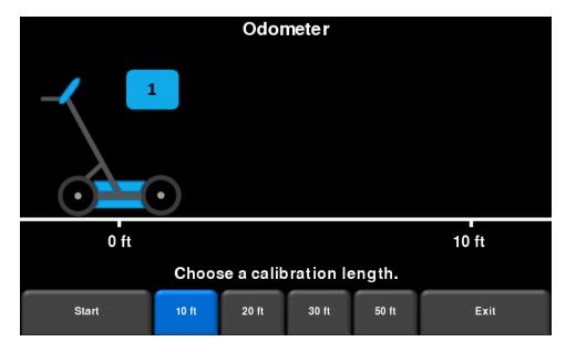
Figure 6-19: Odometer Calibration – select a distance and then press Start
