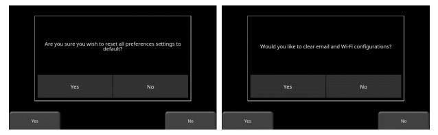
Figure 6-9: Reset to Defaults, a) Image on left is the first confirmation screen. b) If you press **Yes**, you will see the second confirmation screen on the right asking about deleting e-mails and WiFi settings.
