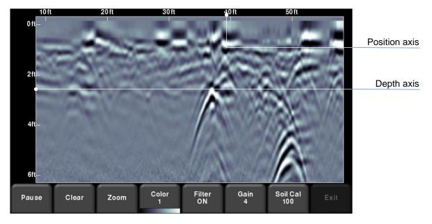
Figure 8-2: Line Scan acquisition mode, showing collected data and axis labels
