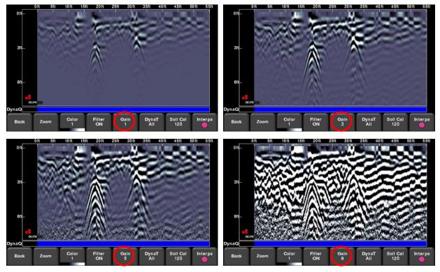
Figure 8-10: Varying the Gain
