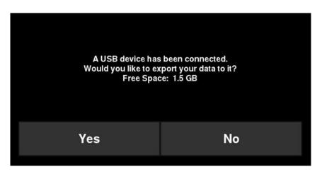
Figure 10-2: When a USB drive is connected to the Display Unit, a message opens asking if you would like to export all your data to it.
