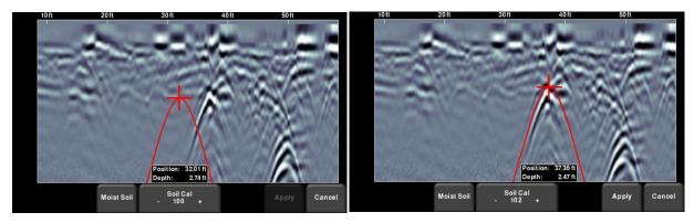
Figure 8-12: Pressing **Soil Cal** displays a red hyperbola (Left). Then move the hyperbola so that it lies over a hyperbola from the ground and adjust the shape (Right)
