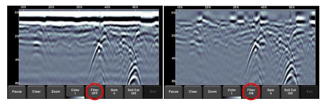
Figure 8-9: Left image shows Filter Off, while the right shows the same data with the Filter On
