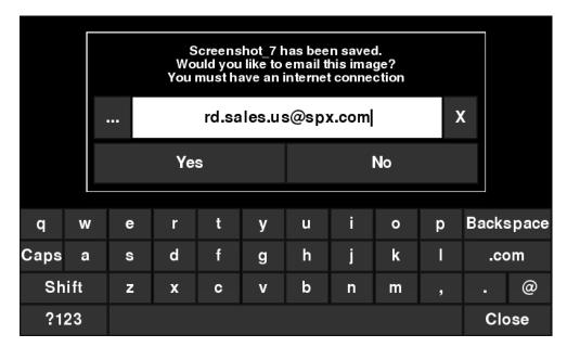
Figure 9-2: Message after pressing the Camera button on the Display Unit to capture the screen with WiFi enabled and a connection to a wireless network. The user can enter an email address to send the mini-report to
