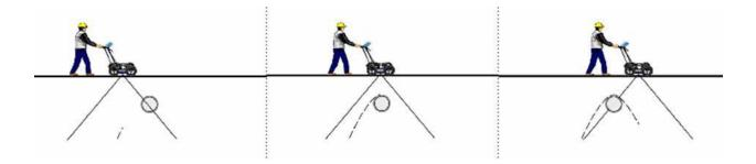
Hyperbolas are best viewed when subsurface targets are crossed perpendicularly or at a 90degree angle. The actual position of the object is located at the apex of the hyperbola.
