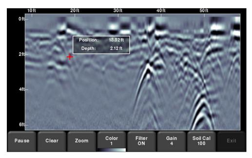
Figure 8-4: Touch screen to get depth and horizontal position at any point
