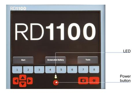
Figure 5-1: Front of Display Unit
