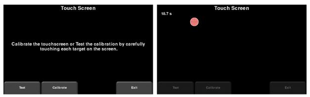
Figure 6-14: Touch Screen test on the left, Touch Screen calibration test on the right
