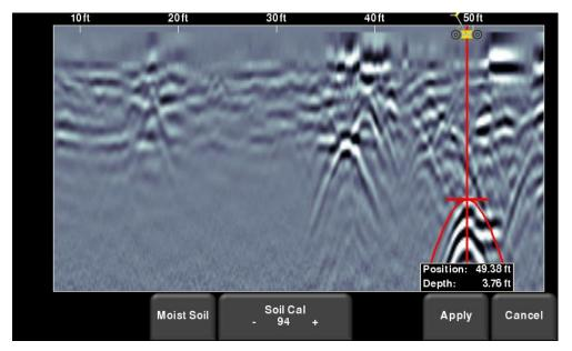
Figure 8-11: Adjusting Soil Cal while in backup mode
