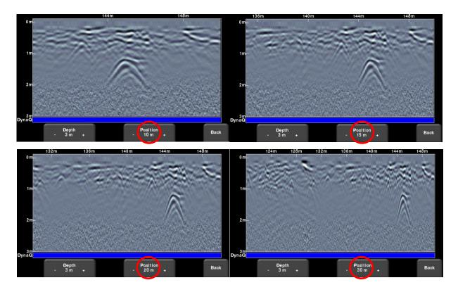
Figure 8-7: Varying position, or horizontal scaling
