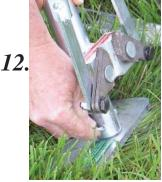
**VERY IMPORTANT:** If you are pulling a stake from a stake bar or frame plate, put the metal base of the lacklaw unit **ONTOP** of the bar or plate. You must pull the stake straight out of the bar or plate. If the unit is on the ground next to the bar or plate, a slight misalignment can cause the stake to bind with the bar, making it difficult to pull from the bar.
